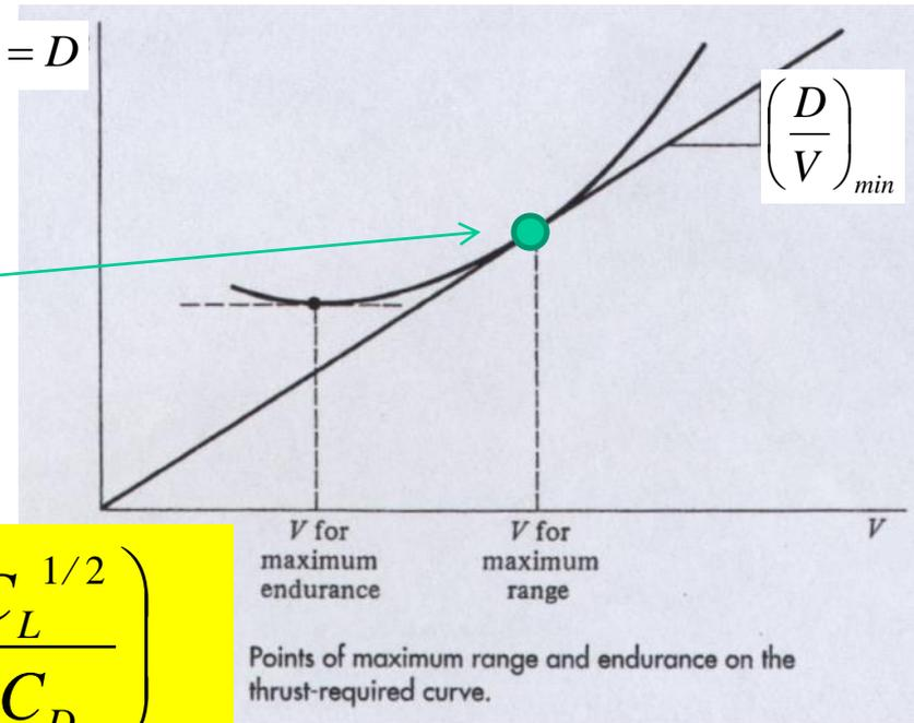
$$\left(\frac{D}{V}\right)_{min} \Rightarrow (E \cdot V)_{max} \Rightarrow \left(\frac{E}{\sqrt{C_L}}\right)_{max} \Rightarrow \left(\frac{C_L^{1/2}}{C_D}\right)_{max}$$
