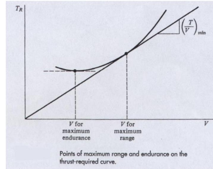
$$\text{Quindi : } \frac{D}{V} = \frac{W}{E} \frac{1}{V} = W \frac{C_D}{C_L} \sqrt{\frac{\rho}{2}} \sqrt{\frac{S}{W}} \cdot \sqrt{C_L} = \sqrt{\frac{W \cdot S \cdot \rho}{2}} \cdot \frac{C_D}{C_L^{1/2}}$$
